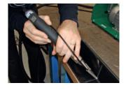
The small hand tool for welding of thermoplastic materials for plastic fabricators. Air supply with external blower (BAK-Air Station) or compressed air.
