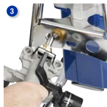
Use frame hex fitting to loosen pump and remove cartridge
