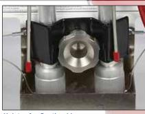
Holster for Suction Lines Keeps tubes in place during transport; prevents drips.
