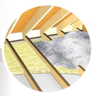
Use the Reactor E-8p in attics to create an air barrier under blown-in insulation (above), or to seal and insulate rim joists (below).
